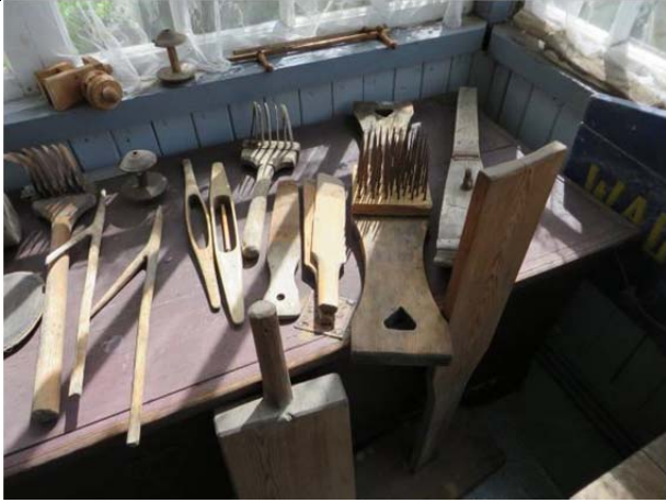
Various historic tools used in converting flax plant into fibers for linen cloth in Latvia. Photo courtesy of D. Ceplis.
